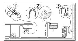
The waste connection must be at a height of between 30 cm (minimum) and 100 cm (maximum) from the bottom of the dishwasher.
